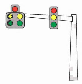
The flashing yellow left-turn signal is in both the State of California's and the Federal Highway Administration's (FHWA) Manual on Uniform Traffic Control Devices (MUTCD). These publications set the standard for signs, signals, and pavement markings in California and the United States. FYA left-turn phasing has been successfully installed in the City of Petaluma, City of Santa Rosa, Town of Winsor, and other jurisdictions throughout California.
