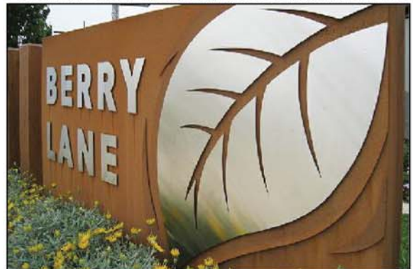
CORTEN STEEL WITH STAINLESS OVERLAY EXAMPLE
