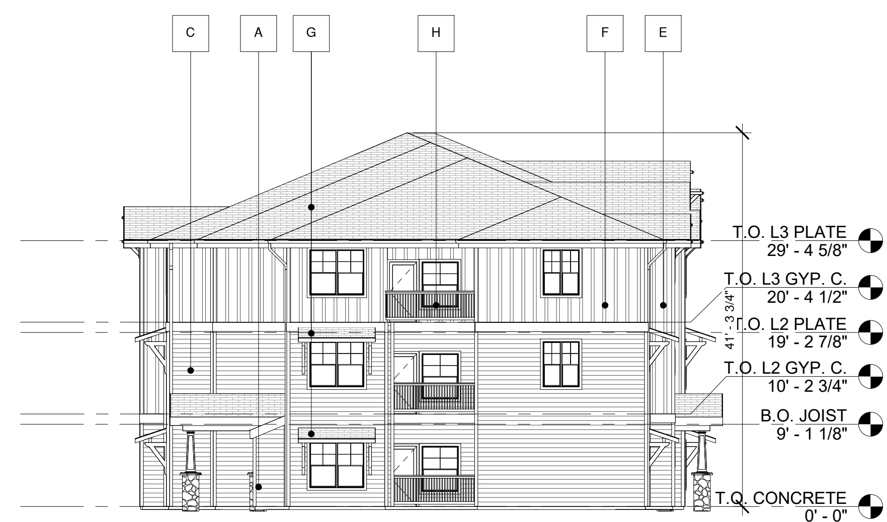
2 LEFT ELEVATION - BLDG. TYPE A 3/32" = 1'-0"
