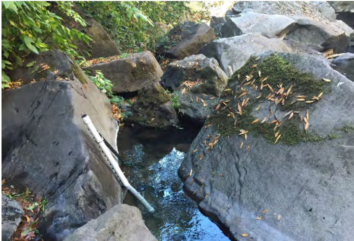
Figure 1: Pressure transducer to be installed at Iron Canyon to measure flows.
