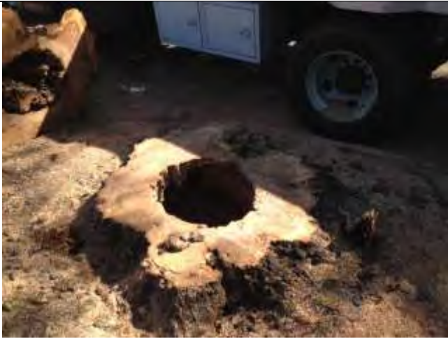
Figure 37. The decay becomes more extensive below ground.
