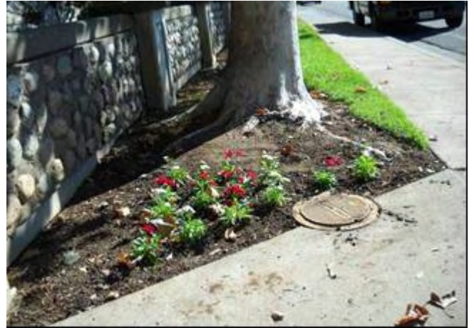
This sycamore tree in the F:2 position was planted 3 feet away from a PG&E gas line that is only 24 inches below ground.
