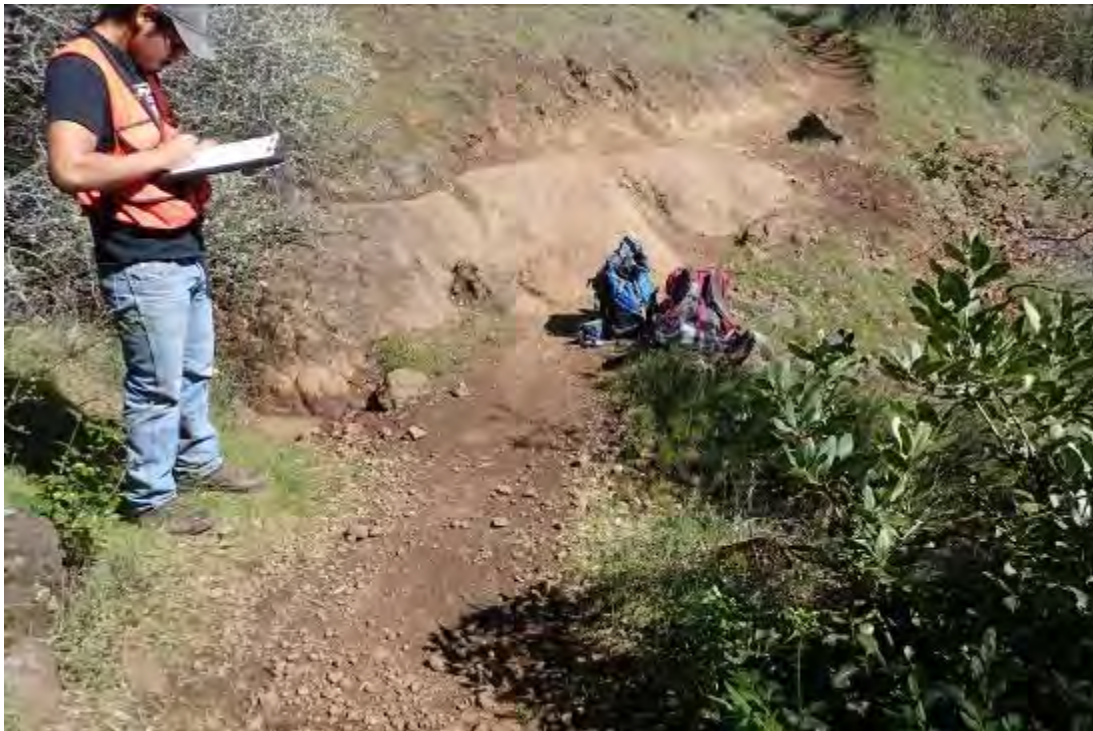
Photo 2. View of PWA Geologist completing the erosion assessment and site inventory data form on the B-Trail. Trail use and trail erosion have exposed bedrock and delivered fine sediment to this ephemeral stream crossing during storms (Site #109).
