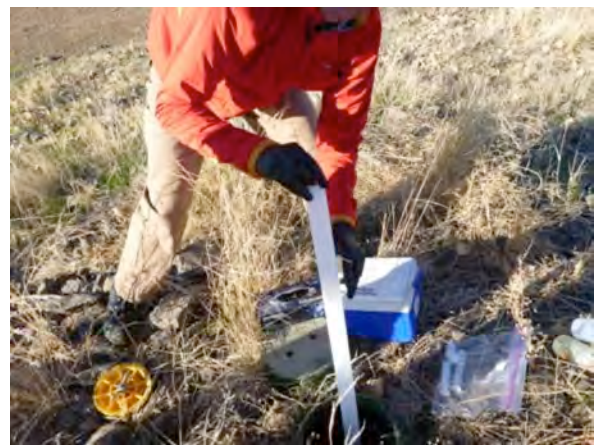
Photo 6: The vault contained three inches of stagnant water, and was sampled for total lead, dissolved lead and hardness.
