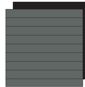
D FIBER CEMENT 9" LAP SIDING TO MATCH BENJAMIN MOORE "DOWN PIPE" 26 BY FARROW & BALL
