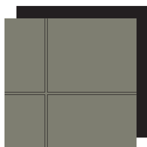
B CEMENT BOARD WITH 1/2" PAINTED METAL REVEALS, COLOR TO MATCH SHERWIN WILLIAMS "LINK GRAY" SW 6200
