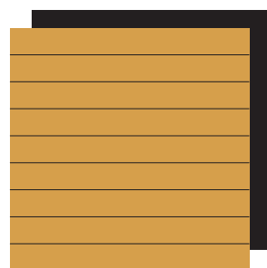
E 8.25" SMOOTH CEMENT BOARD LAP SIDING, COLOR TO MATCH BENJAMIN MOORE "APPLE CRISP" 2159-30
