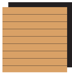
E 8.25" SMOOTH CEMENT BOARD LAP SIDING, COLOR TO MATCH SHERWIN WILLIAMS "HARVEST GOLD" SW 2858
