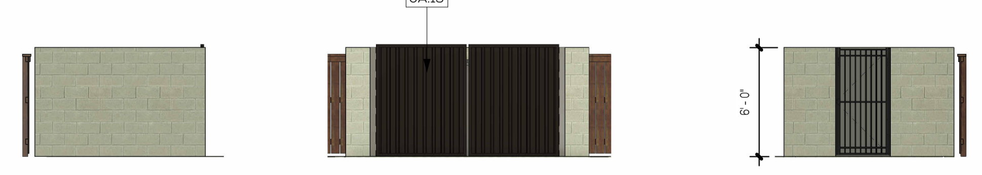
5 - TRASH ENCLOSURE ELEVATIONS SCALE: 3/16" = 1'-0"
