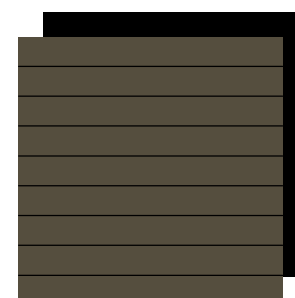
D 8.25" SMOOTH CEMENT BOARD LAP SIDING, COLOR TO MATCH SHERWIN WILLIAMS "ENDURING BRONZE" SW 7055
