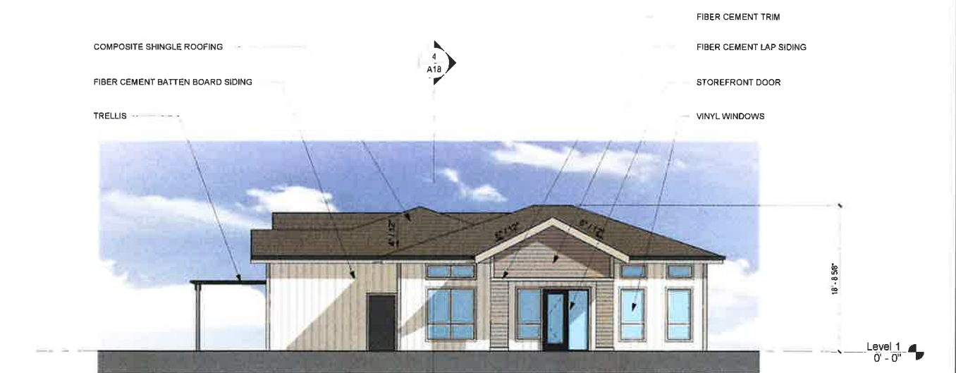
COMMUNITY BUILDING - SOUTH ELEVATION 1/8" = 1'-0" 2
