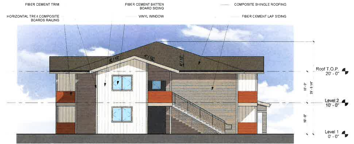
BUILDING 7- SOUTH ELEVATION 1/8" = 1'-0" 3
