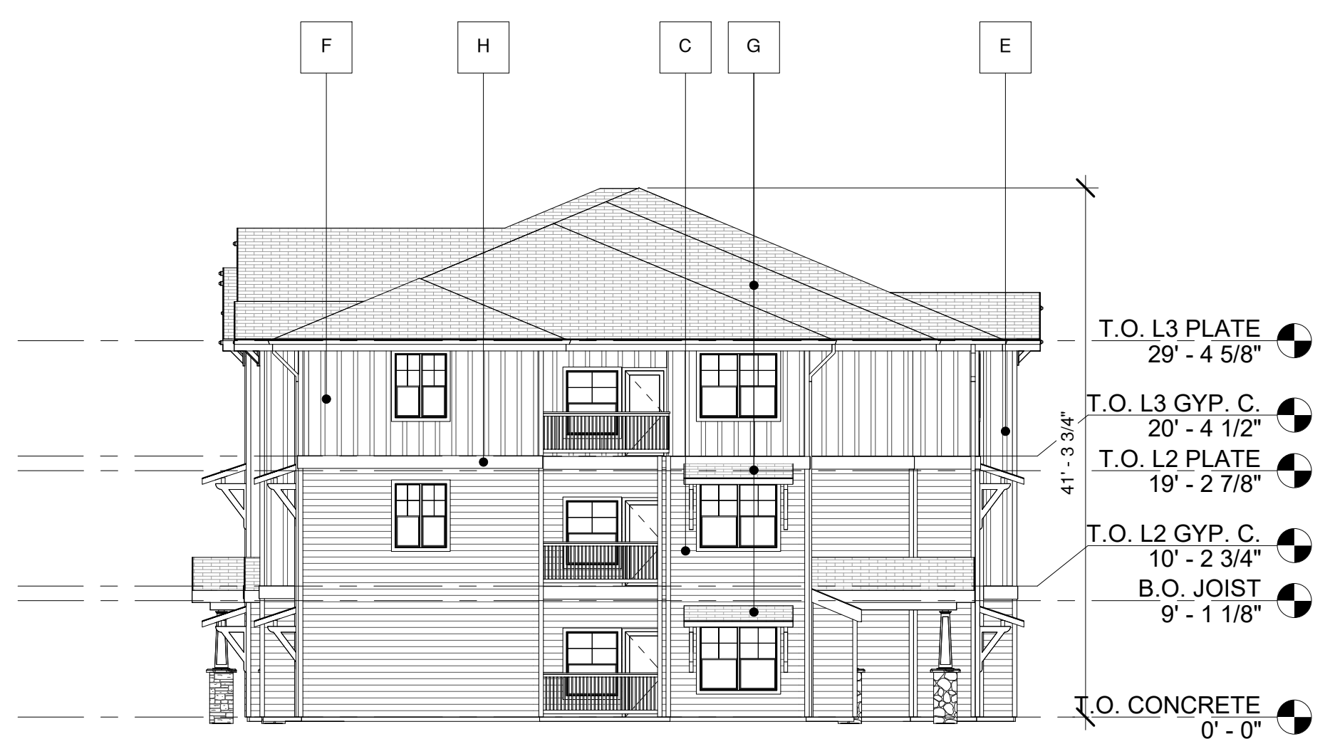
3 RIGHT ELEVATION - BLDG. TYPE A 3/32" = 1'-0"
