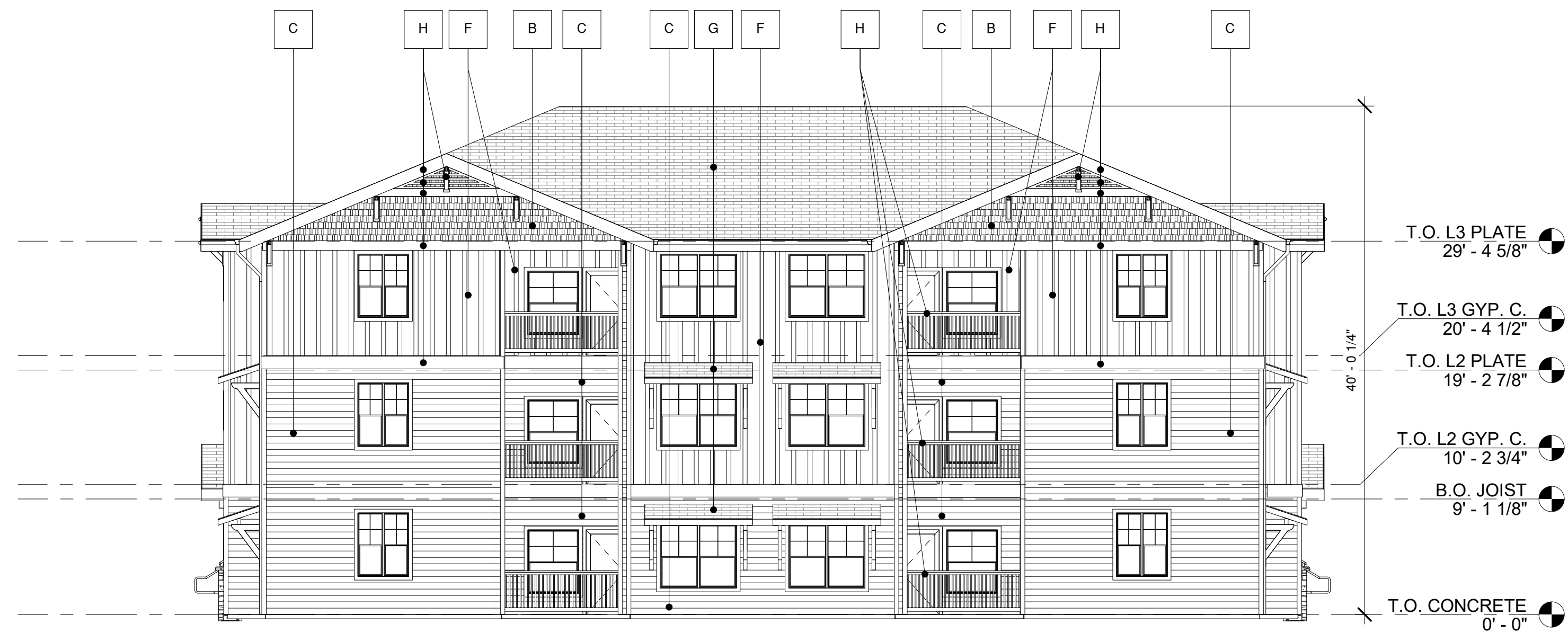
1 FRONT ELEVATION - BLDG. TYPE B 1/8" = 1'-0"
