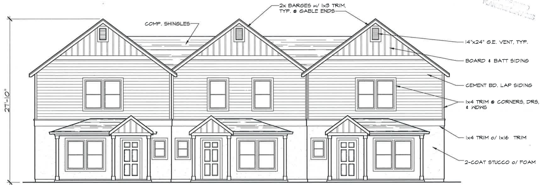
FRONT ELEVATION (EAST AND WEST ELEVATIONS) 1/8" = 1'-0"
