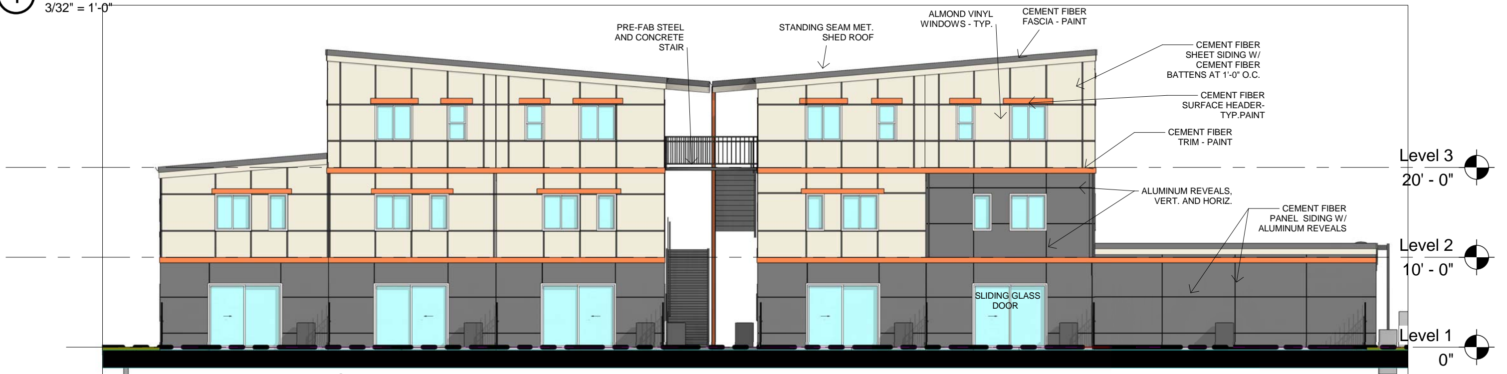
2 North Elevation - Bldg. One 3/32" = 1'-0"
