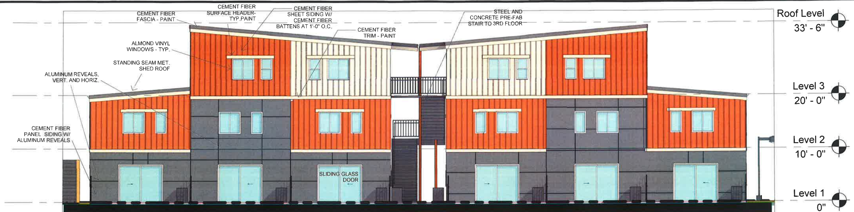
BUILDING 2 - NORTH ELEVATIONS 11X17
