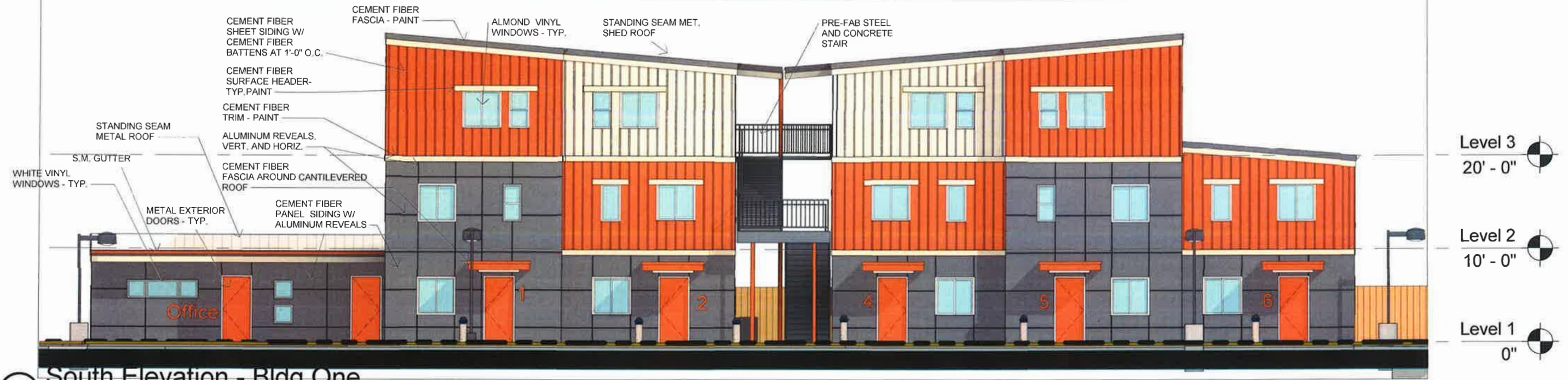
1 South Elevation - Bldg One 3/32" = 1'-0"
