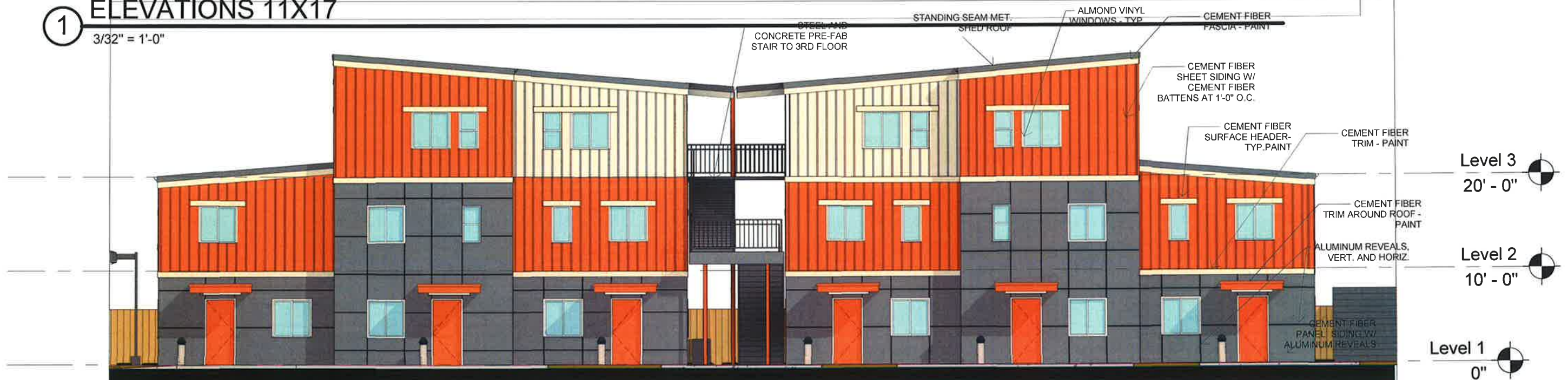
BUILDING 2 - SOUTH ELEVATION 11X17
