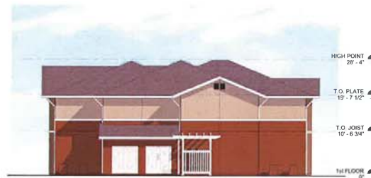
12 UNIT (TYPE A) BUILDING EXTERIOR ELEVATION | 1 12'-7 1/2"
