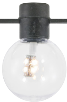
12V LED Festoon Socket Assembly 3000K / 1.5W / 80,000hr rated life Black base; max run = 300W LFS-12V-1.5-LED-WW 1.5 watts
