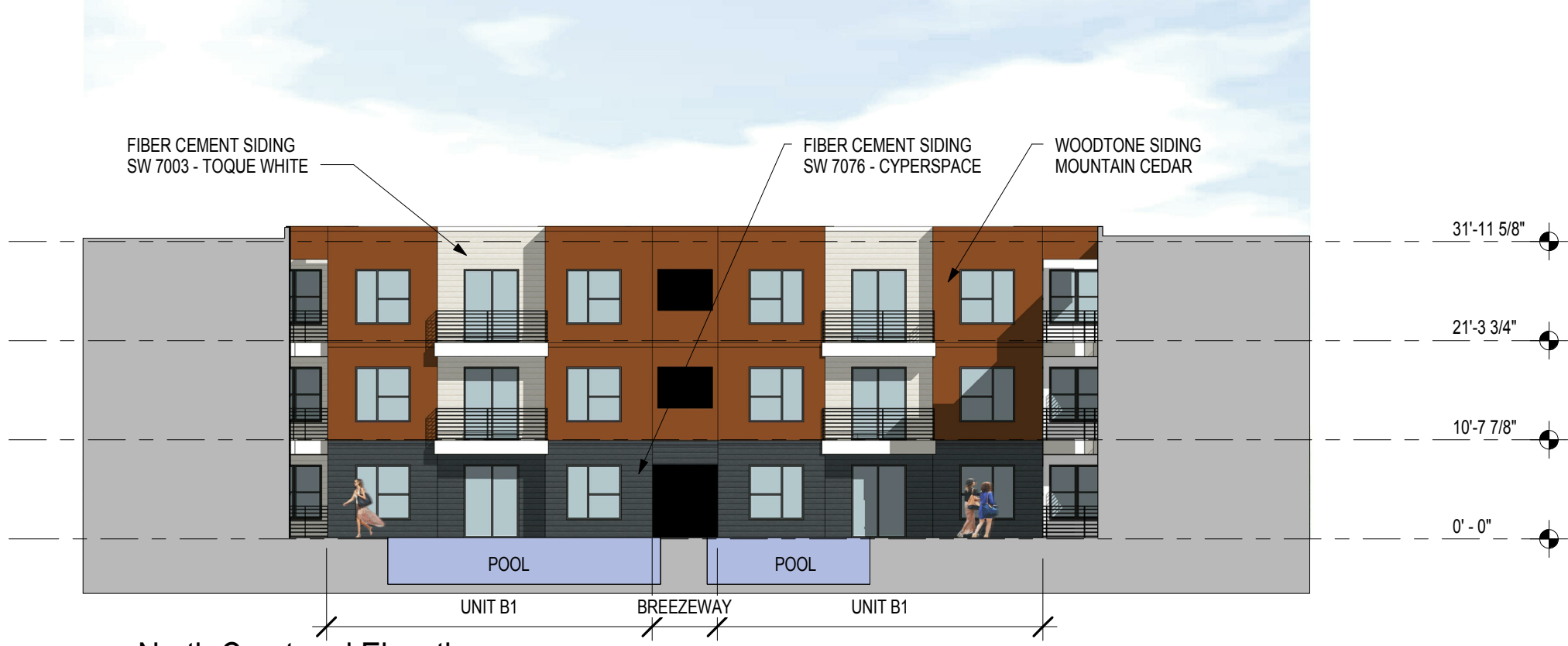
2 North Courtyard Elevation 1/16" = 1'-0"
