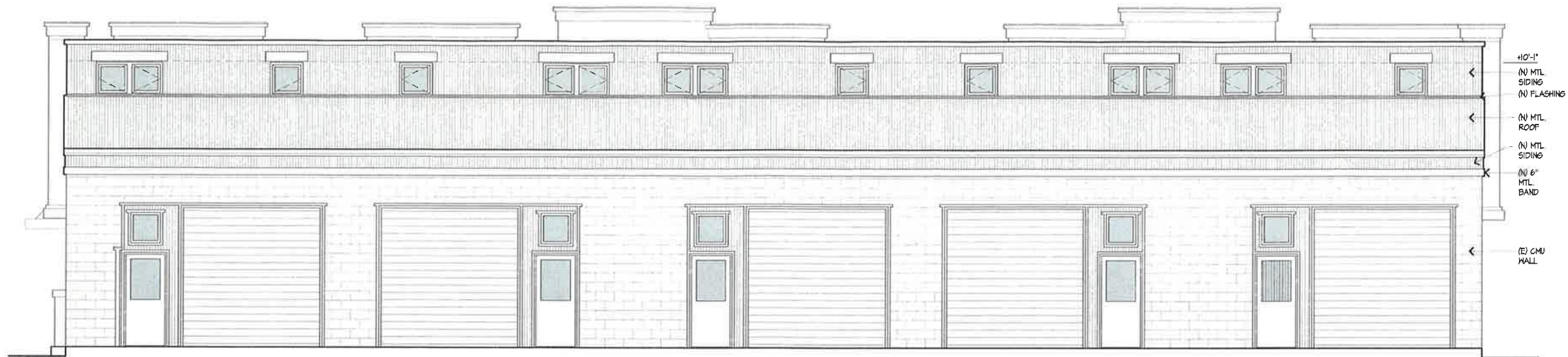
REAR ELEVATION SCALE: 1/4" = 1'-0"
