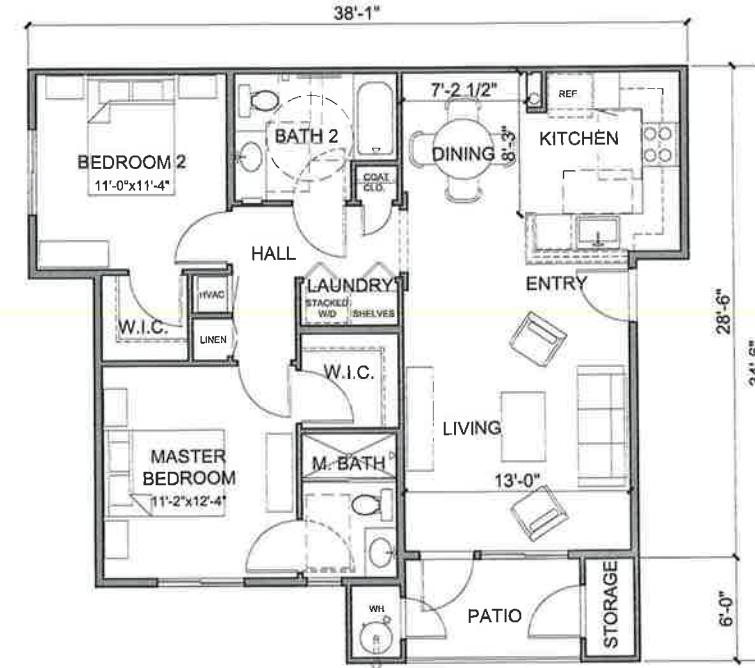
UNIT A1 - 2 BED / 2 BATH LIVING: 999 SF. STORAGE CLOSETS: 36 SF. PRIVATE PATIO: 60 SF.
