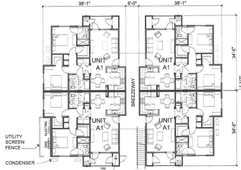
BUILDING TYPE 1 - 1ST FLOOR 2ND FLOOR SIMILAR
