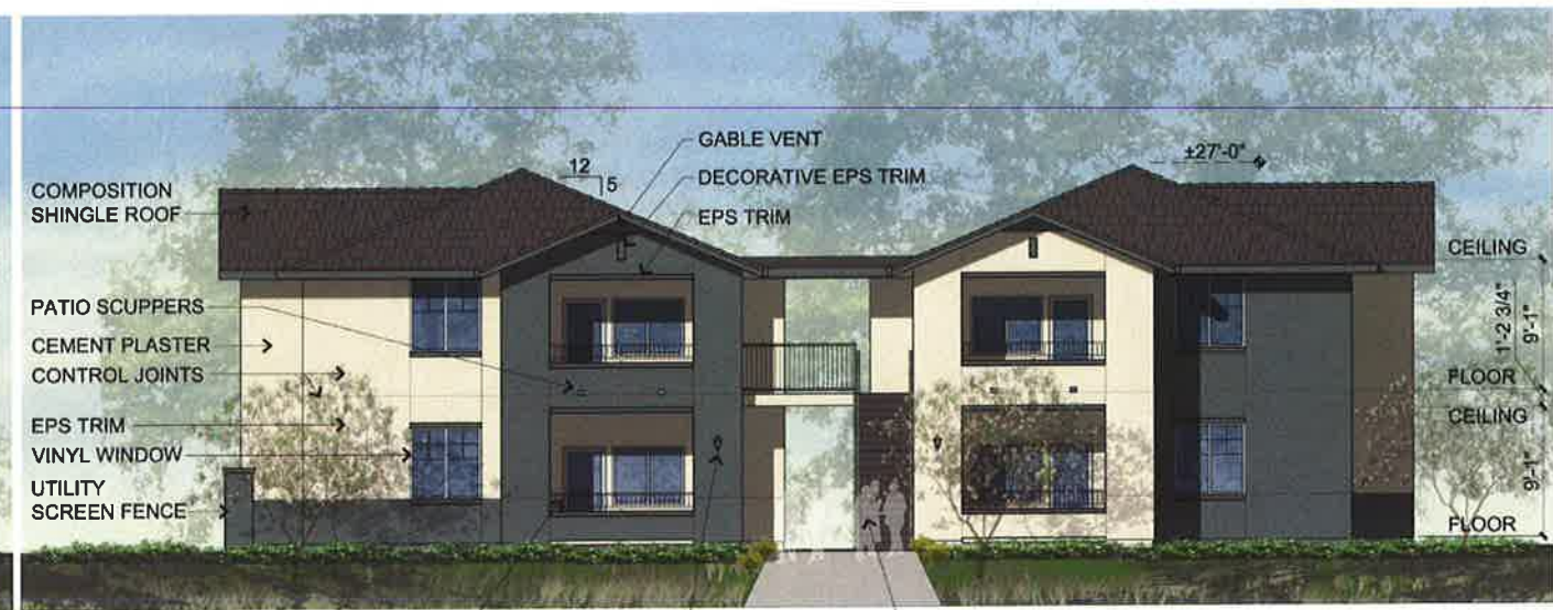
FRONT ELEVATION - BUILDING TYPE 2
