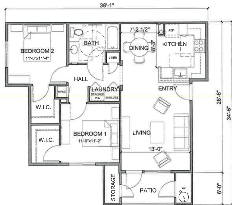
UNIT B1 - 2 BED / 1 BATH LIVING: 929 SF. STORAGE CLOSETS: 47 SF. PRIVATE PATIO: 60 SF.
