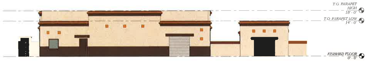
2 SUPPORT FACILITY ELEVATION - EAST SCALE 1/8" = 1'-0"
