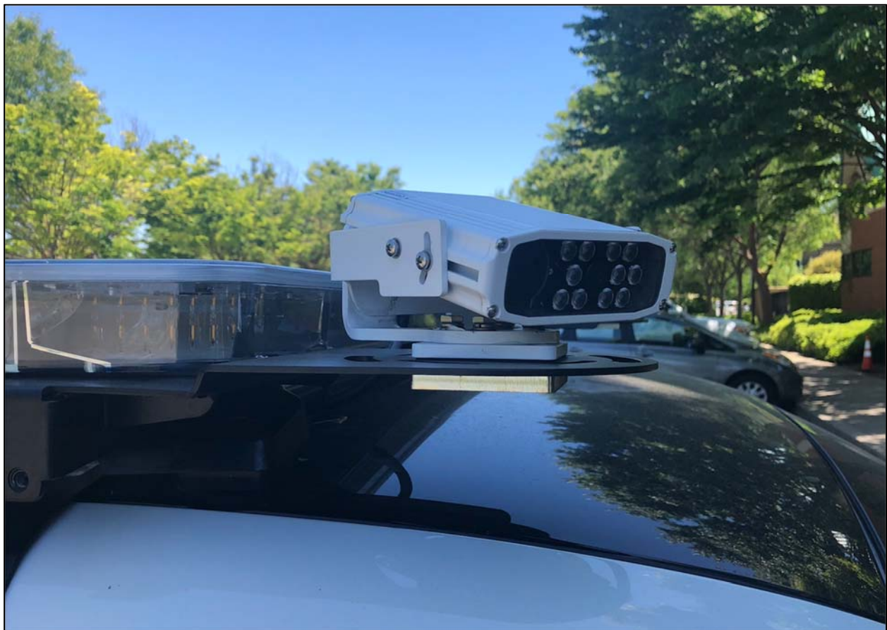
Image 7. LPR Mounted on City of Davis Enforcement Vehicle
