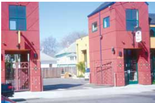
Parking lots should be located behind buildings to enhance the pedestrian character of the street.
