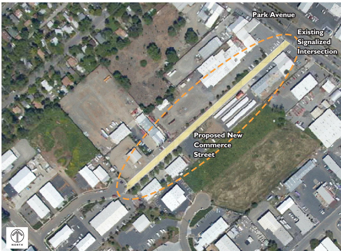
Figure 4-34. Connecting Park Avenue and Commerce Court with a new street along the path of an existing alley to provide a second access to the Meyers Industrial Area.
