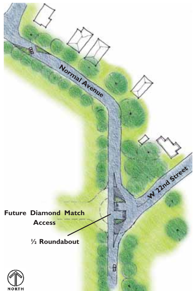
Figure 5-9. Potential Traffic Calming with a half roundabout on Normal Avenue and West 22 nd Street.
