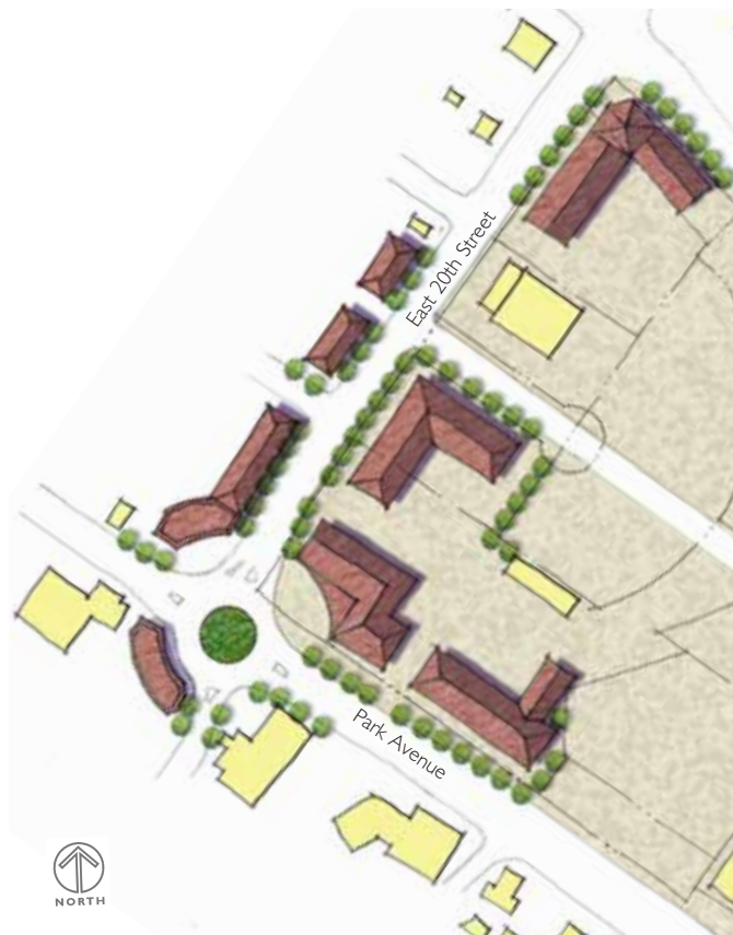
Figure 4-15. Park Avenue at East 20 th Street conceptual plan showing new mixed-use development and a roundabout.
