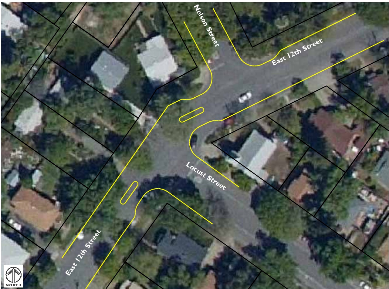
Figure 5-7. Potential Traffic Calming for the East 12 th , Locust, and Nelson Streets Intersection.
