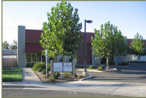
DG 6.1.21- Efficient site design minimizes paved area for parking and truck maneuverability
