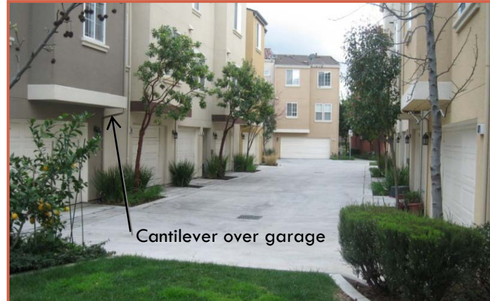
DG 4.1.61- Garages are placed at the rear and share a common driveway
