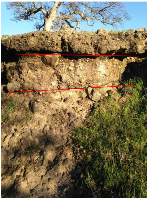
Photo 5: 3 foot thick conglomerate lens beneath 4 foot thick lahar layer at ravine within Section 118. More lahar underlies conglomerate lens, which is of limited lateral extent. Note the rounded cobble in the conglomerate vs the more angular clasts within the lahar.
