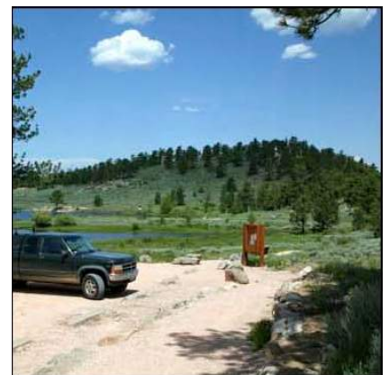
Example parking lot showing clearly marked trail access point. Wheelstops and low boulder wall create use barrier. Adjacent gravel path is provided for trail access.
