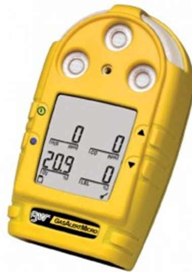
Photo 2. Typical Personal Four-Gas Monitor
