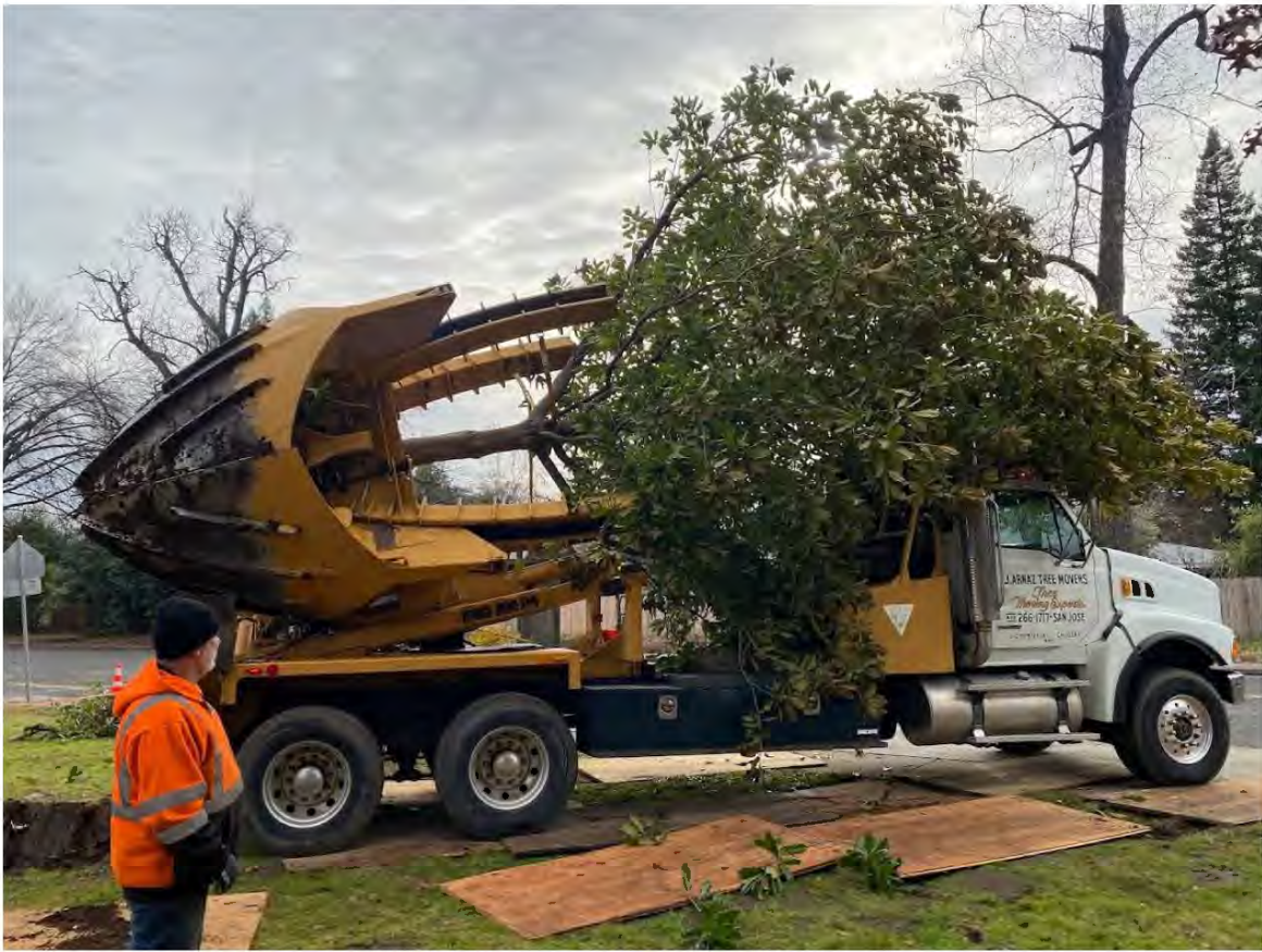
Figure 2: Tree and root ball loaded for transportation to a new location.
